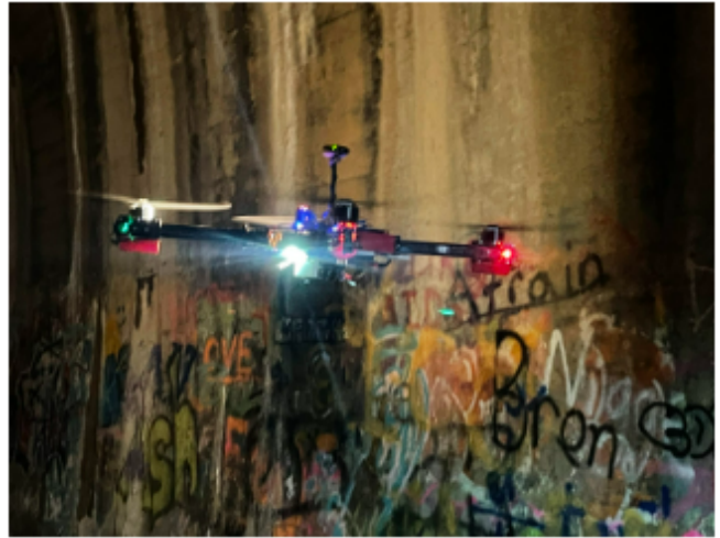
Fig. 13: Full Integration Test of System in the Clinton Tunnel
